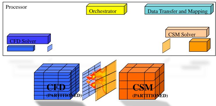
To handle the burning, we need a combustion solver capable of operating on geometry and data from other solvers and their domains.
