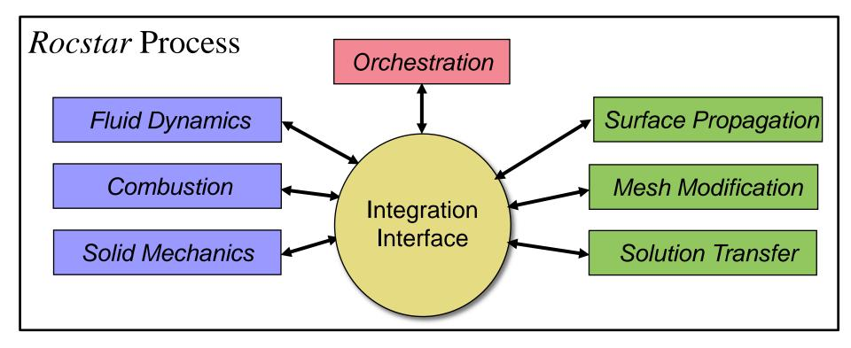
The integration interface provides the mechanisms by which applications can publish and access methods and data. This is the "glue" of the *Rocstar* multiphysics simulation.
