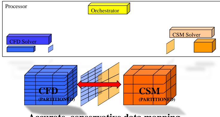
Accurate, conservative data mapping across the interface and processorgeometry mapping is required.
