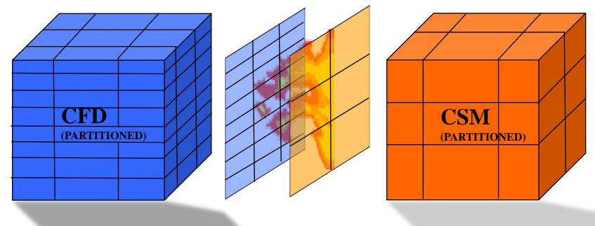
The interface is reactive. It catches on fire, injects materials, and propagates (burns).
