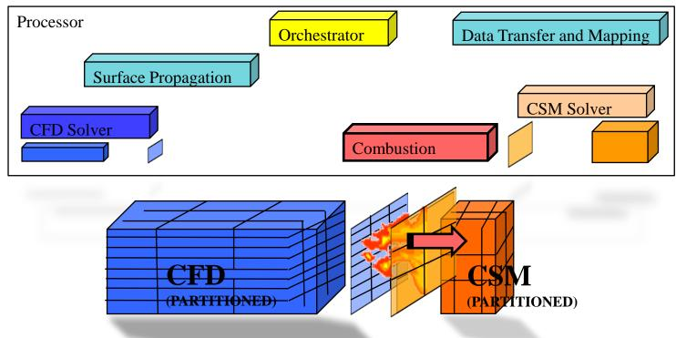
Mesh modification will be required for handling the extreme changes in geometry due to burning and deformations.
