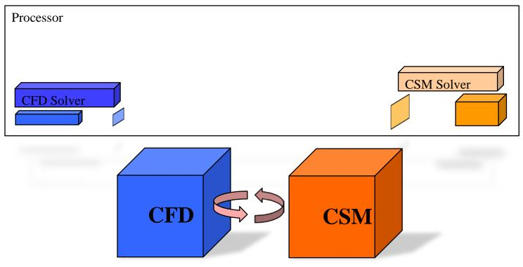
There must be a control flow manager for synchronous stepping, to handle some jump conditions, unit conversions.
